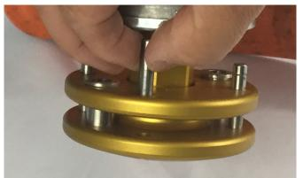
2. With medium in place, lower guide pin to secure. Pin is magnetically held in place. There should be resistance when lifting pin. When lowering, there should be a snapping in place with an audible click. If pin is not firmly in place, repeat process. If problem still exists, do not use and contact support.
