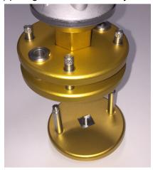
Next, locate 1/4 serrated lock nuts and install on threaded post using 1/4 wrench to tighten.
