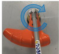
Direction is defined by rotation observed when holding trimmer in normal operating manner as shown CW in picture. For units with CCW rotation, the Flat
